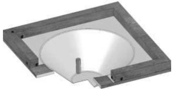
Fig. 1. Single Point Incremental Sheet Forming
